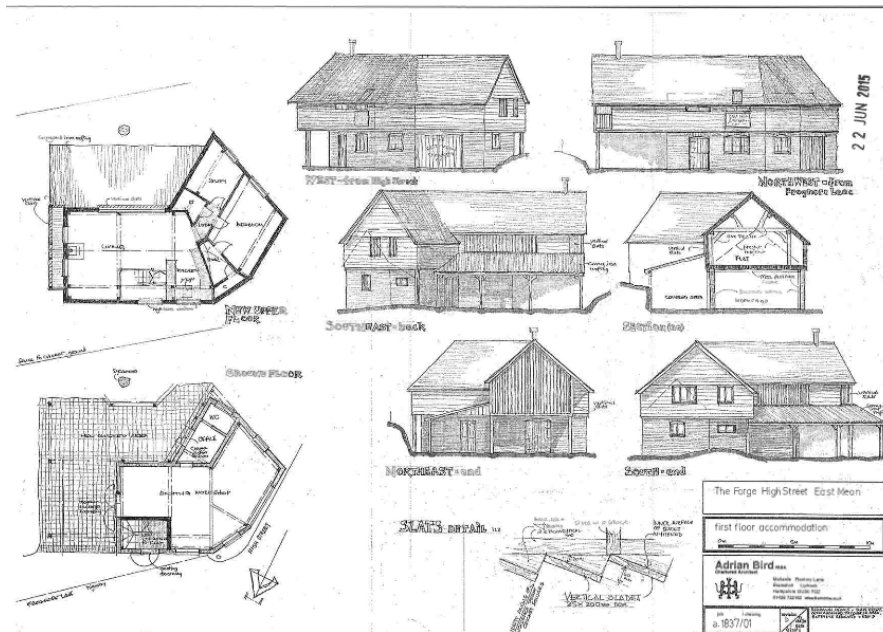
Revised plans for re-development of The Forge. The design included an open deck on the south-west side, facing the cricket pitch..
